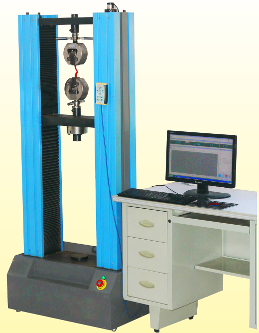
Tear strength testing equipment
