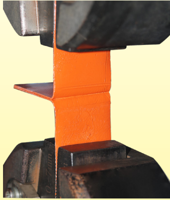
Vulcanized sample before decoupling test
