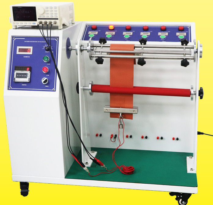
Flexible silicone heater during the flexion test
