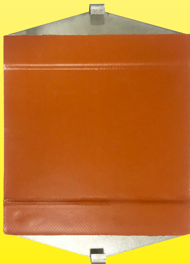
Tear force testing sample
