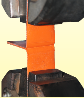
Vulcanized sample before decoupling test
