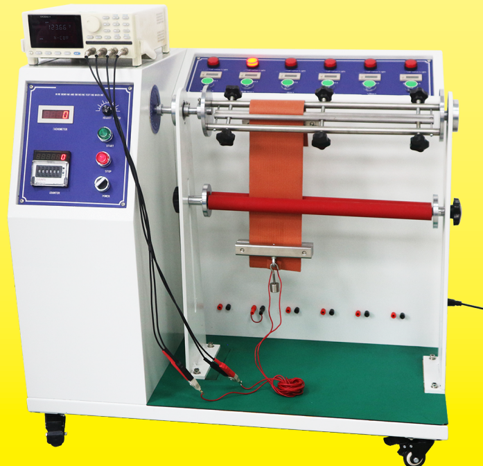
Flexible silicone heater during the flexion test
