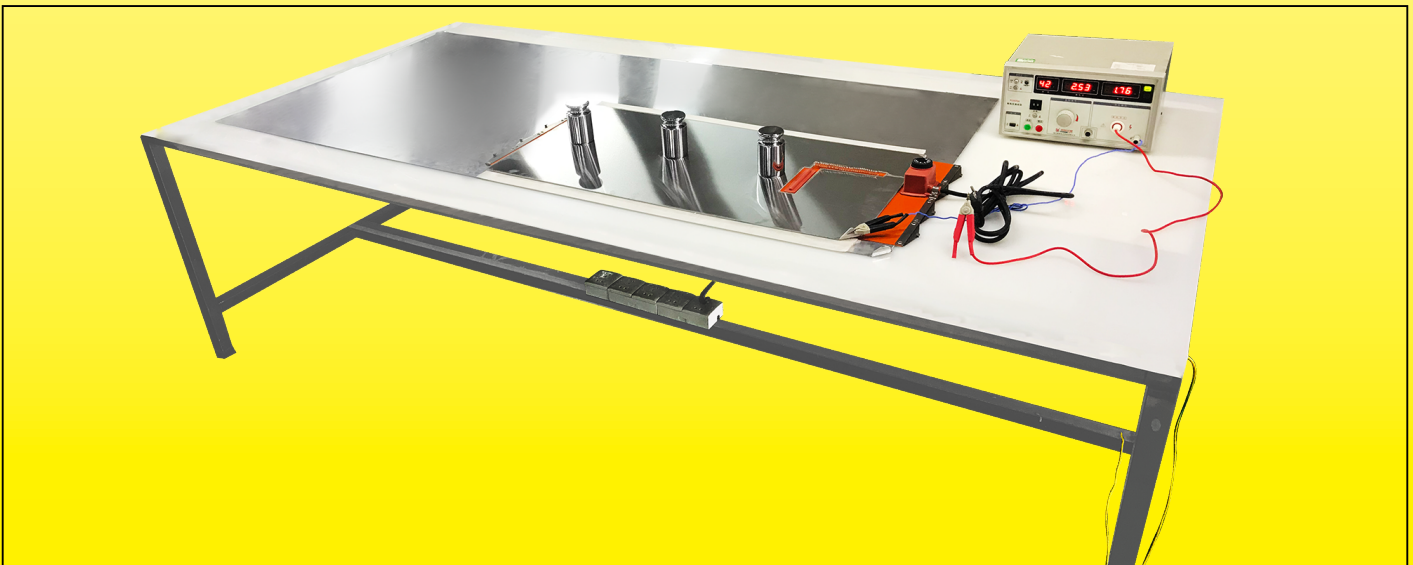
Measuring equipment for total current leakage at cold condition
