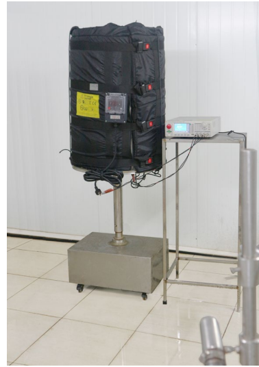
Insulation resistance measurement after IPx6 tests
