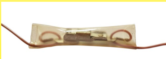
Calor slow-break heating blanket temperature limiter, calibrated at 80°C (circa 1960). Note the waterproof PVC sleeve welded on the wires and the loop made by the electrical conductors passing through a hole in each terminal- this is to eliminate tensile stresses on the wire (Ultimheat Collection)
