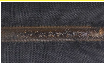
1h at 235^{\circ}C on the heating cable: The PA66 begins to melt
