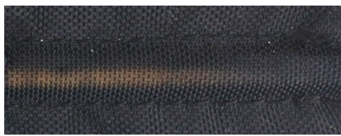
1h at 220^{\circ}C on the heating cable: the PA66 starts to change color
