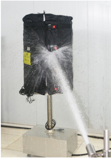
IPx6 testing of jacket heaters
