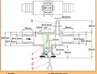
Main uses:Tee equipped with paddle flow switch, for spas and swimming pools applications, mounting on 1" (20 to 21mm ID) soft PVC tubes, adjustable setting.
