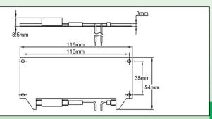
Immediately below the level of the transparent window, the warm air flow it generates prevents from condensation on the window and keeps an optimum ambient temperature for the control devices in the housing. It has a wide aluminum heat exchanger to reduce its surface temperature and a miniature snap-action thermostat limits the temperature inside the cabinet.
