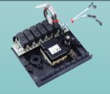
6 relays 16A 250V on thermostat extended front board, with single pole thermostat
