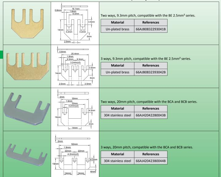
These shunts are used to connect two or three terminals of standard power terminal blocks. They do not prevent from connecting other conductors to the terminals. They are accessible by the end user or installer.
