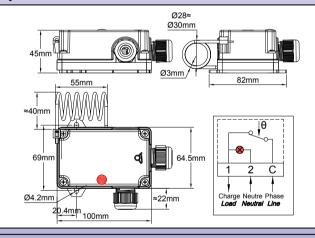
Example of wall mounting model connected on Y25 connection boxes for antifreeze protection of livestock waters
