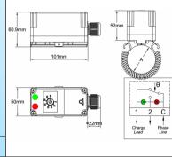
This thermostat is designed with a V shaped temperature sensitive nickel plated brass backside to improve thermal contact with the pipe, and two lugs for spring mounting. Suitable for pipes of 30 to 70mm diameter.
