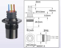
3 wires Pt100 sensor in an anodized aluminum bolt. For temperature control of a pipe surface: to be screwed on the mounting stand. The length of the conductor outputs allows direct connection into the control box via the M20 rear outlets, if this component is mounted on the same stand:
