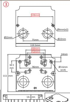
Aluminum board. For customer drilling and mounting.
