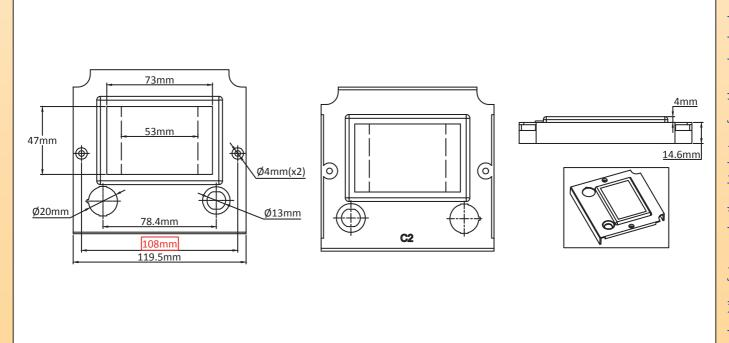
PA66, one rectangular hole 73x47mm. With two mobile caps for reduce and move hole to 53x47mm. Can be used for 2DNA and ground fault detection contactor. Hole for on-off switch and hole for fusible holder. No studs for relays or contactors. When used with 2DNA, fits flat cover enclosures.
