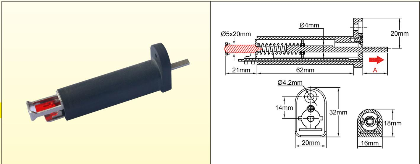
These mechanical thermal actuators are intended to close the fire dampers used on the ventilation ducts. Their **large operating force unlocks the spring actuating the damper**. Requiring **no power supply**, these devices are particularly simple and reliable. They are mandatory for all fire dampers to meet the NF-S 61.937 standard. **Since thermal bulbs are not subject to creep, their periodic replacement is not necessary.**
