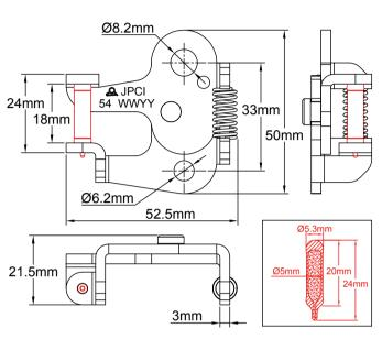
Made of 3mm thick galvanized steel, these reduction mechanisms are compatible with 20x5mm thermal glass bulbs. Their huge multiplying coefficient reduces the force applied to the thermal glass bulb to only 15% of that applied to the mechanism. The replacement of the glass bulb is simple and can be done without special tools.
