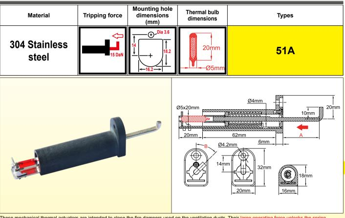
These mechanical thermal actuators are intended to close the fire dampers used on the ventilation ducts. Their large operating force unlocks the spring actuating the damper. Requiring no power supply, these devices are particularly simple and reliable. They are mandatory for all fire dampers to meet the NF-S 61.937 standard. Since thermal bulbs are not subject to creep, their periodic replacement is not necessary.
