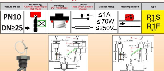
Main uses: The most simple flow switch with magnetic pull-back. Recommended mounting position is on horizontal pipes, but can be mounted in any position. For water 25 to 63 mm water pipes.
