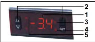
**Control:** Two independent heating zones, each of them controlled by a simple to use electronic thermostat with digital display (1) and set point adjustment (2) from -45°C to +120°C (41~248°F); They use NTC sensors. (Main features: Adjustable differential; 0.1 ° resolution up to 99.9; °C (3) or °F display (4); parameters locking function, Power supply on and output on pilot lights (5).
