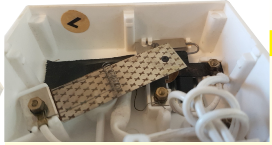
1970 ca. GEC power setting (General Electric, England) on an English heating blanket. Anticipated resistance is clearly visible above the bimetal and slow breaker (Ultimheat Collection).
