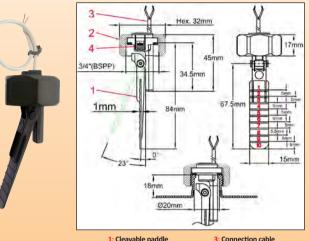
3: Connection cable 4: Adjustment screw 1: Cleavable paddle 2: 3/4" BSPP plastic union nut
