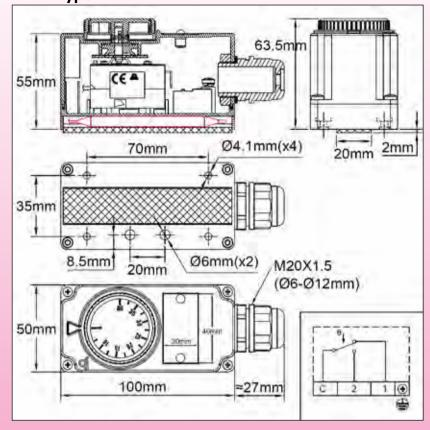
Housing: IP65, 100 x 50 x 75 mm, PC-ABS, 20%FG, UL94V0. High impact and UV resistance, with silicone waterproof gasket on thermostat shaft.
